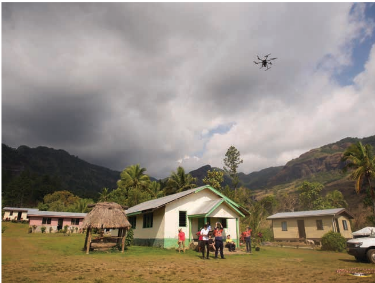
FIGURE 12. Launch of a multirotor UAV, which requires less open space than for a fixed wing.
