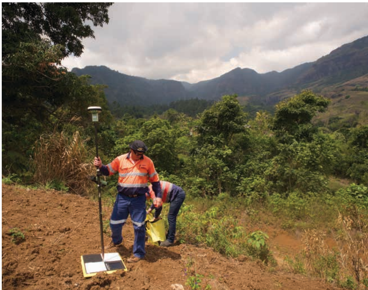
FIGURE 10. Placing of a ground control point. The accurate coordinates of this GCP are surveyed on the spot using high-accuracy GPS.
